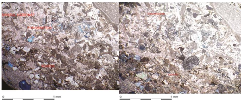
**Figure 8.** Thin Cutlet of Reef Limestone
