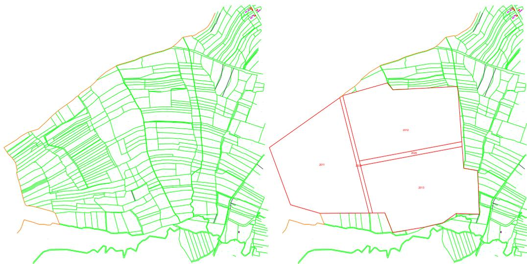
Figure 4: Cadastre situation example before and after the completion of regulation project
