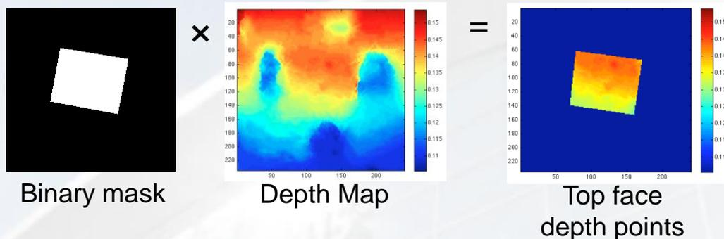
Given that those points are not coplanar, the proposed resolution is to estimate the best fitting plane by [Least Squares Adjustment](#), from the selected depth values.
