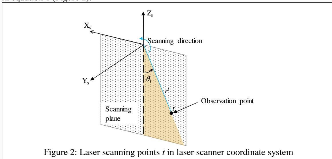
Figure 2: Laser scanning points  $t$  in laser scanner coordinate system
