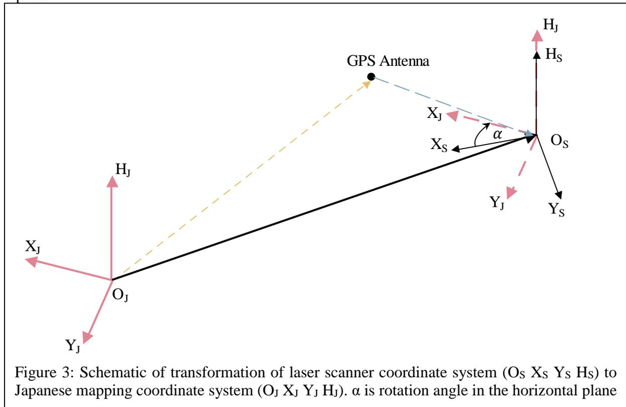
Figure 3: Schematic of transformation of laser scanner coordinate system ( $O_S X_S Y_S H_S$ ) to Japanese mapping coordinate system ( $O_J X_J Y_J H_J$ ).  $\alpha$  is rotation angle in the horizontal plane
