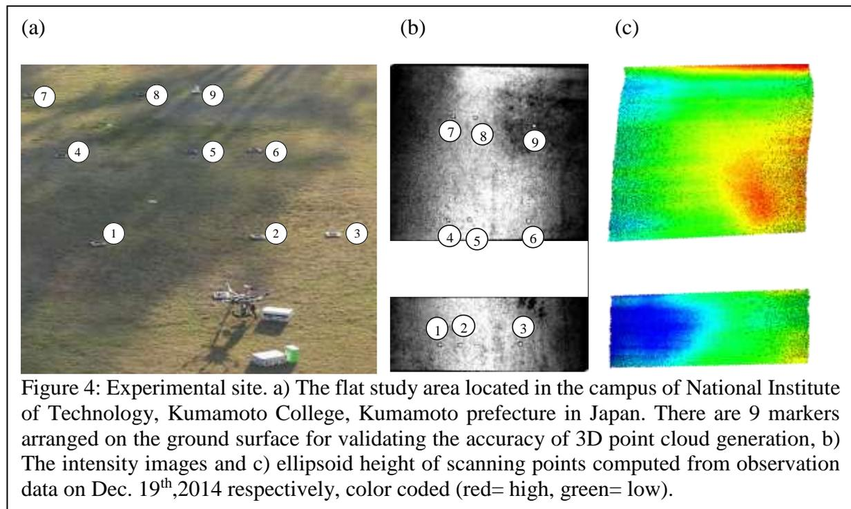
observation data. This coordinate was compared with the coordinated measured by the total station to validate the accuracy of developed system. The accuracy was accessed in two
