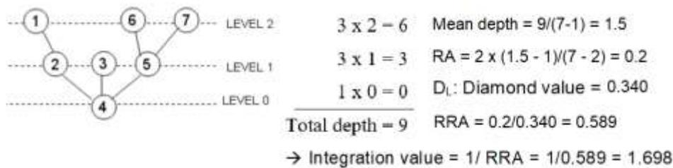
Figure 5. Example of how to calculate the global integration value
