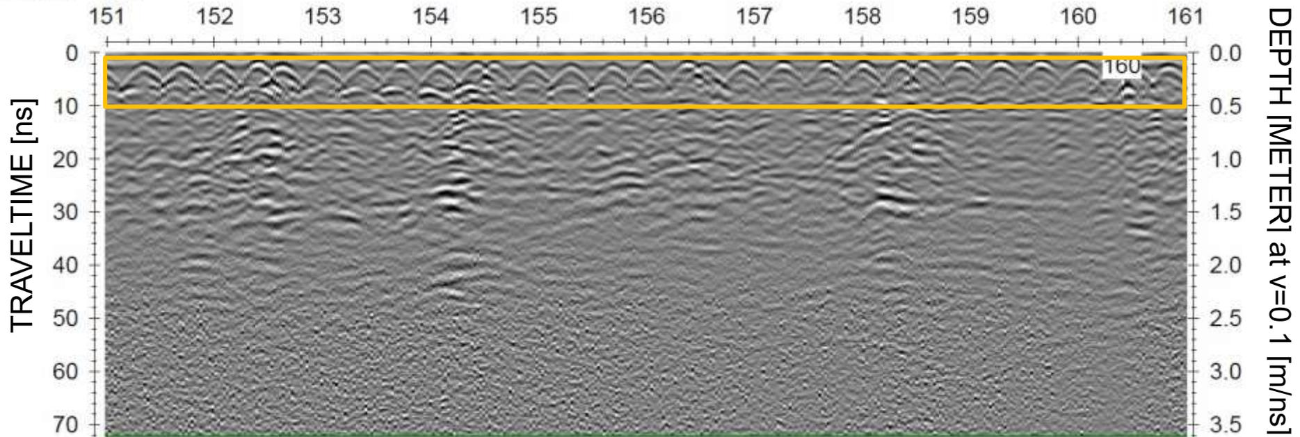
Reinforcing bar's are located at the top of each hyperbola
