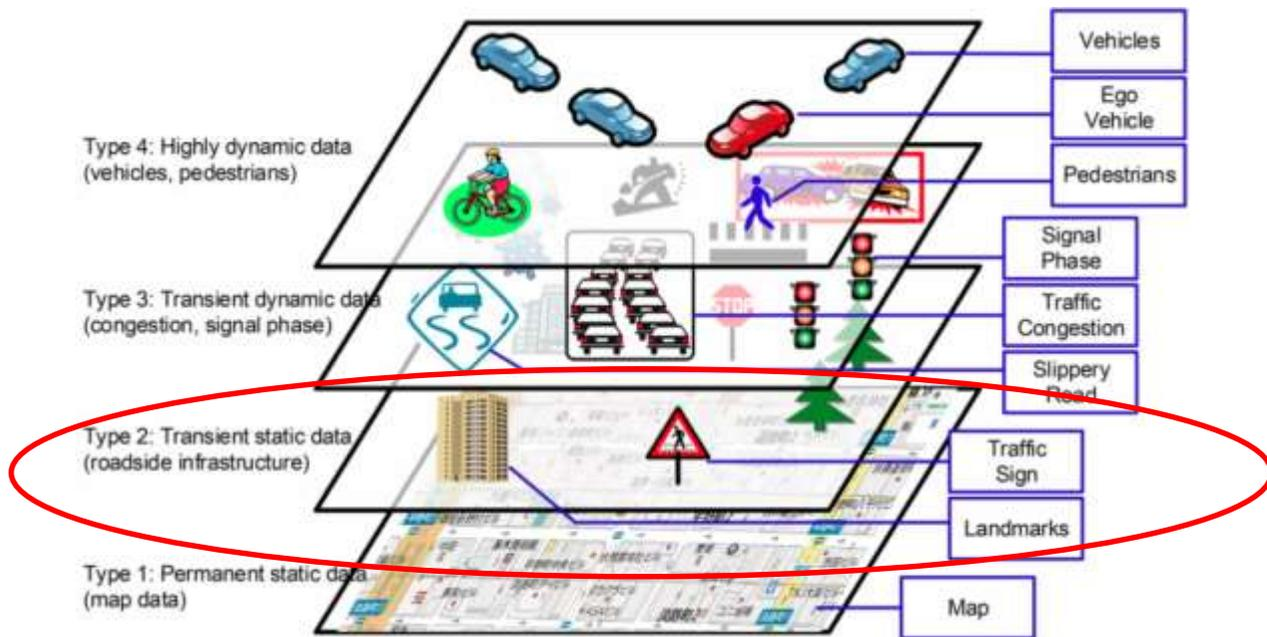
The layered architecture of the LDM (Source: Schimada et al., 2015, "Implementation and Evaluation of Local Dynamic Map in Safety Driving Systems". Journal of Transportation Technologies, 2015, 5, 102-112)
