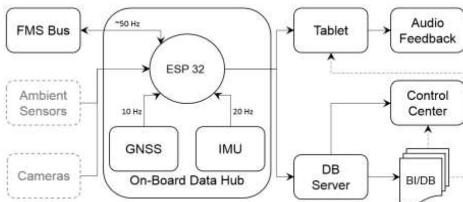
Fig. 1: Data flows and system architecture
