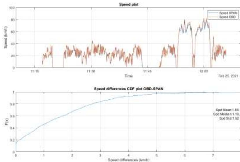
Fig. 10: Speed timeseries and corresponding difference CDF plot
