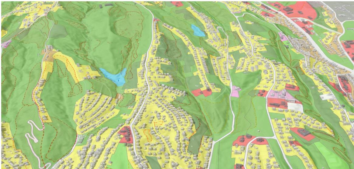
Figure 3. Overlay of land use map, DTM, 3D model and landslide data (Pantovčak, Zagreb)
