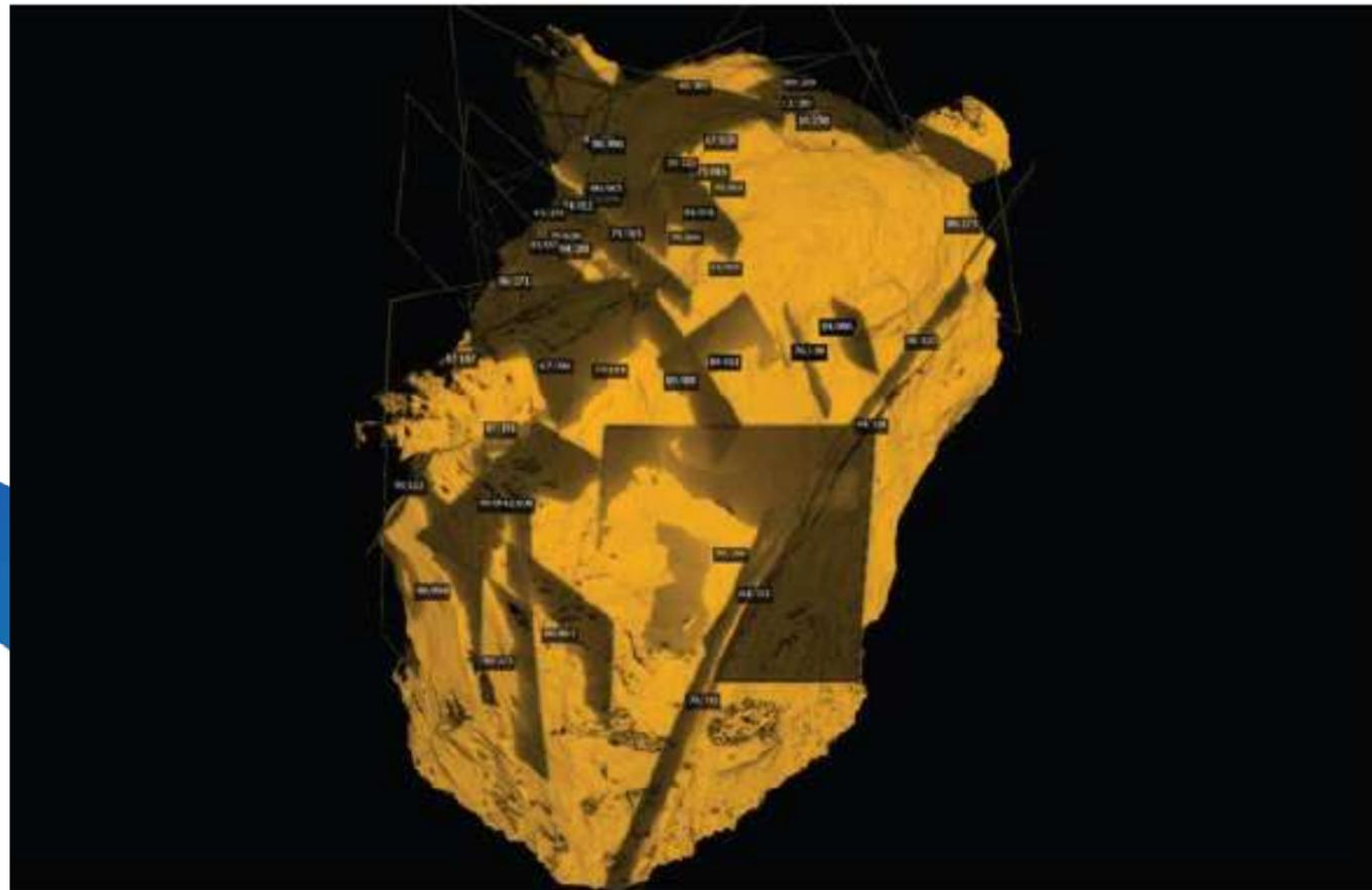
BHP's Olympic Dam mine stoppage analysis process involves picking geological structures from Hovermap scans. High-resolution final stoppage scans are imported into the mine's co-ordinate system before the geotechnical team picks the structures that control the final stoppage shape. (Source: BHP, Evan Jones, Emesent webinar.)
