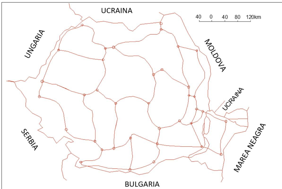
Figure 1 The leveling network of the first order in Romania
