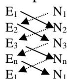
Figure 3: Cross coordinate method of area determination
