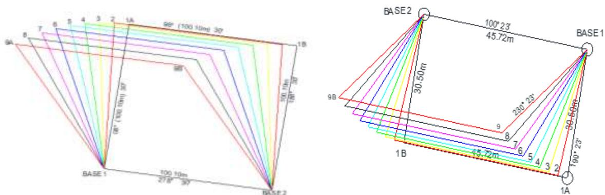
Figure 7: Plans of the different parcels superimposed on each other (100x100m) and (30x45m)
