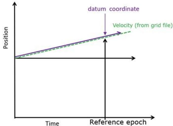
Figure 12 Displacement model with only a constant velocity
