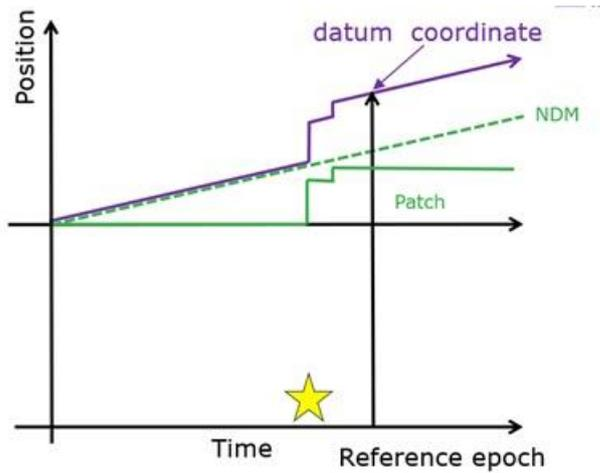
Figure 23 Schematic diagram of a dynamic datum. Dashed green line shows the secular velocity solid green line shows the co-seismic contribution to the displacement model. The solid purple line shows the displacement model with both contributions combined.
