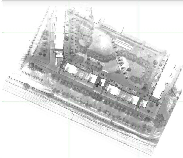
Figure 2: An example of fast extraction of a 2,5D point cloud orthophoto of a complex of buildings
