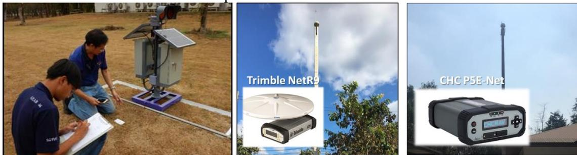
**Figure 8** The low-cost RTK GNSS receiver unit on a linear rail obtaining correction data from the nearest CORS; either Trimble NetR9 or CHC P5E-Net CORS.
