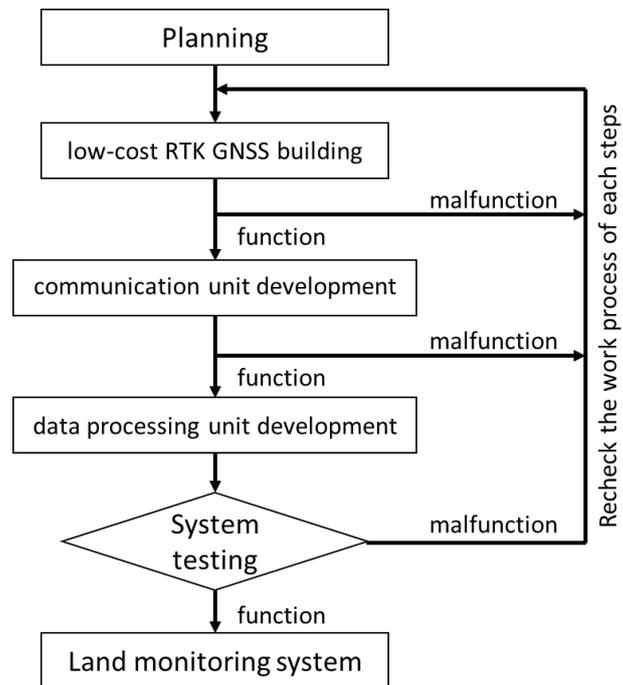
**Figure 3** The procedure of the RTK-GNSS landslide monitoring system, RTK-LANDMOS.
