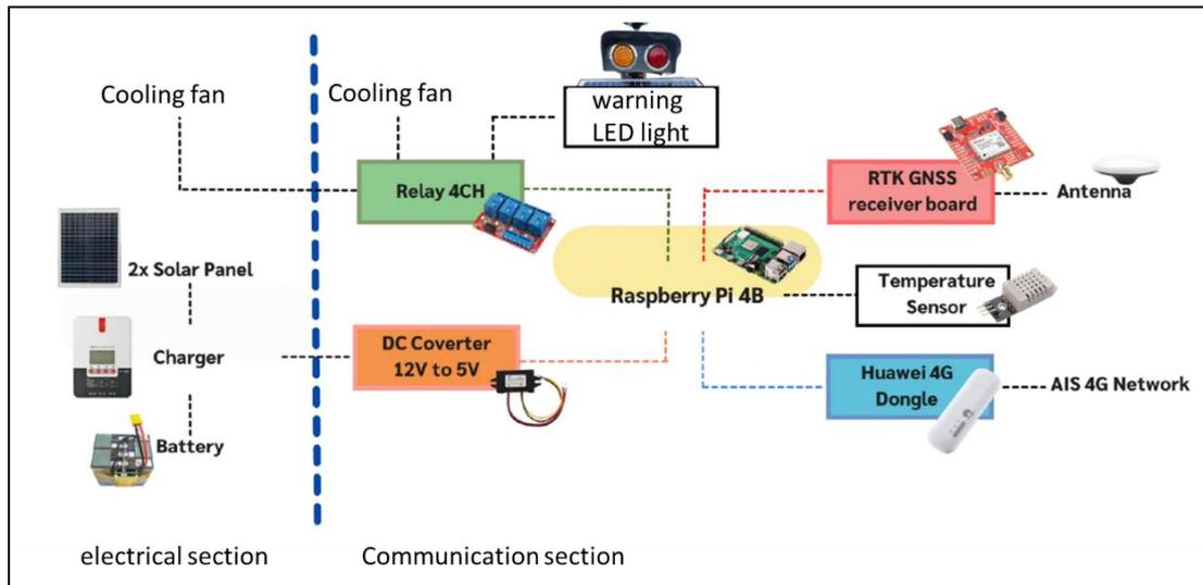
**Figure 4** The components of the built-in low-cost RTK GNSS receiver units.
