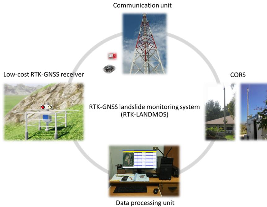
**Figure 2** The architecture of the RTK GNSS landslide monitoring system, RTK-LANDMOS.
