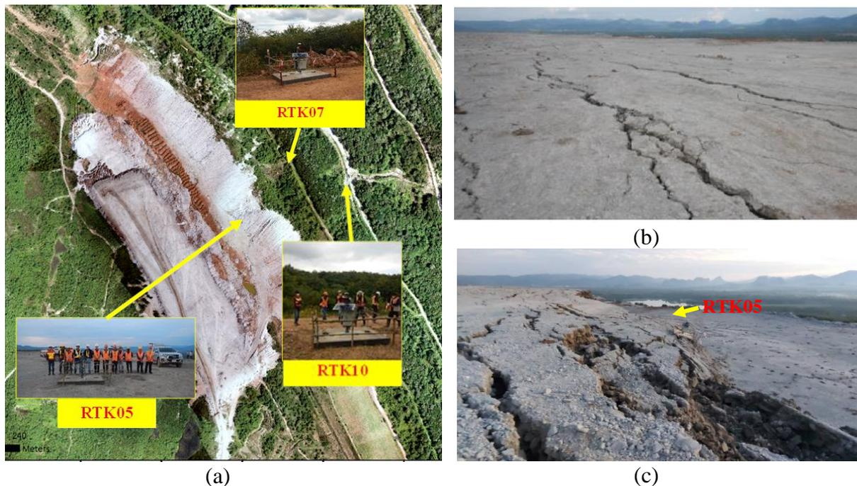
Development of Landslide Monitoring System by Real-Time Kinematic Survey: Experimentation and Application in Mae Moh Mine, Thailand (1973)
