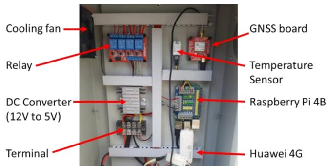
**Figure 5** The example of electronic equipment in a waterproof sheet steel wall box.
