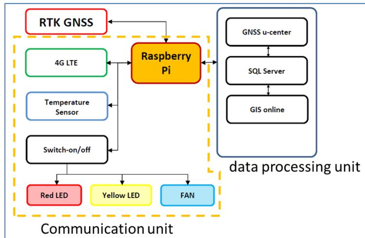
**Figure 6** The diagram of the RTK-LANDMOS structure.
