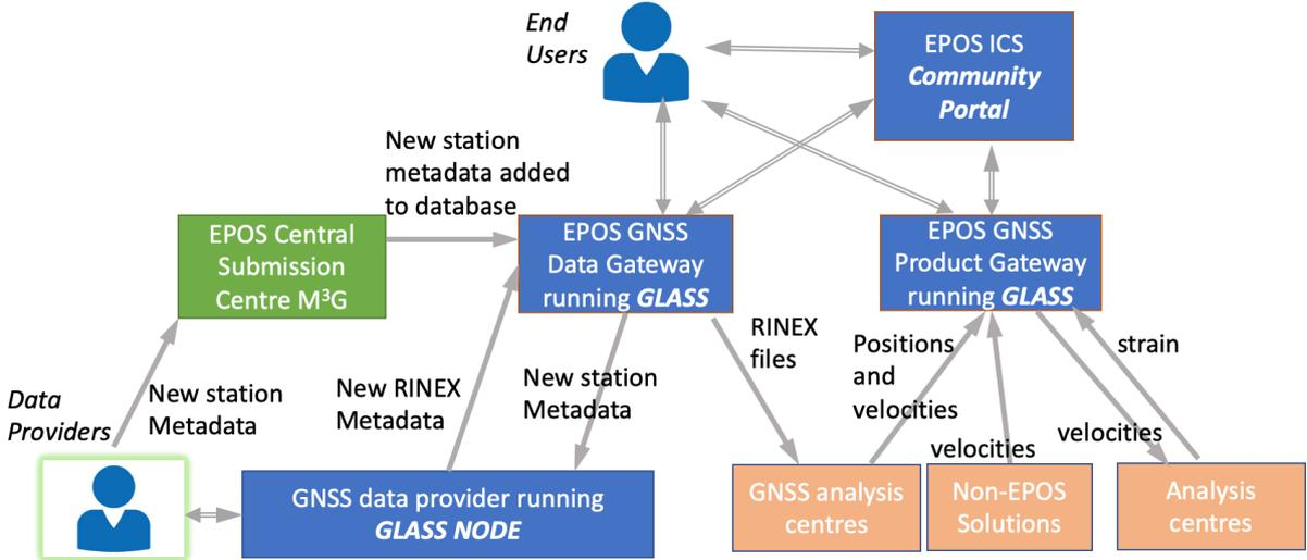
Figure 3 – Data Flows within the EPOS-GNSS framework as seen by a Station Manager and End User
