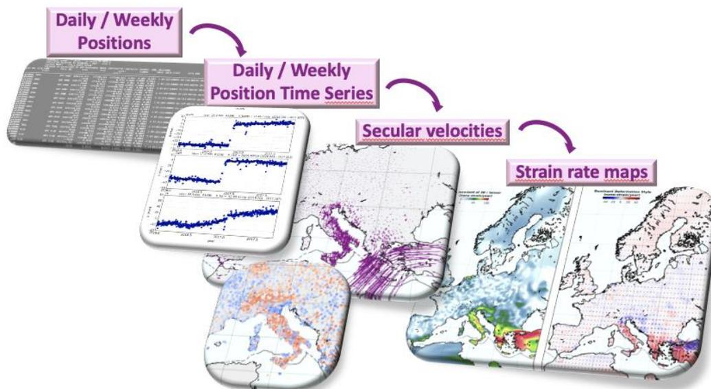
Figure 6 – GNSS products generated and distributed through EPOS-GNSS Products Portal: SINEX files, position time series, secular velocities, strain rate maps
