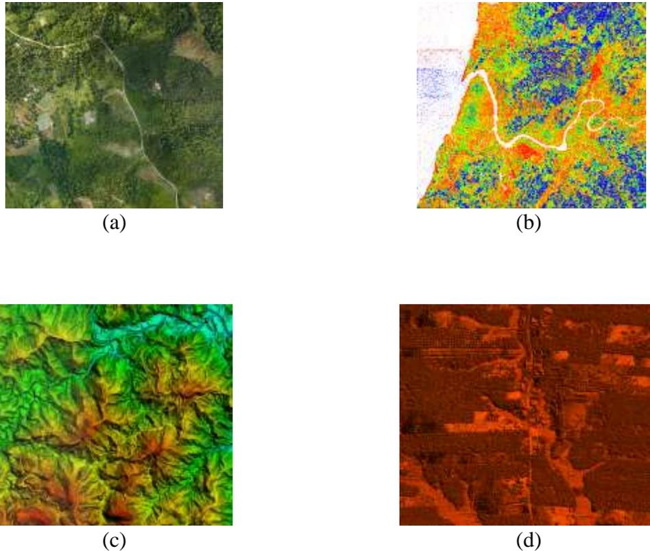
Figure 14. (10a) Aerial Imagery from Airborne LiDAR, (10b) 3D Point Cloud already classified, (10c) Digital Terrain Model (DTM), (10d) Digital Surface Model (DSM)
