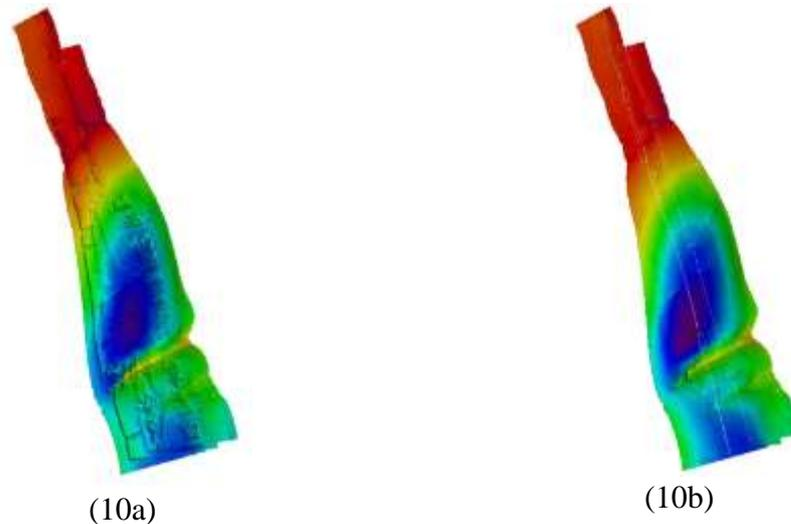
Figure 10a and 10b. (10a) Seafloor DTM before Patchtest Calibration (10b) Seafloor DTM after Patchtest Calibration
