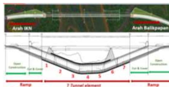
Figure 2. Plan View and Longitudinal Section of Sepaku Immersed Tunnel
