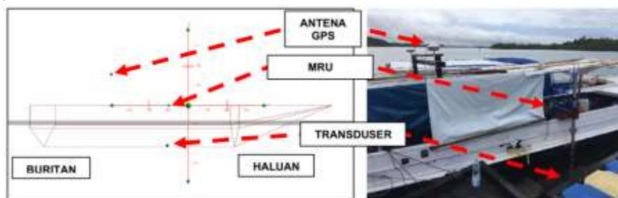
Figure 8. MBES Lever Arm Configuration
