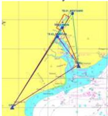
*Figure 7. Baseline Configuration for GNSS Observation*
