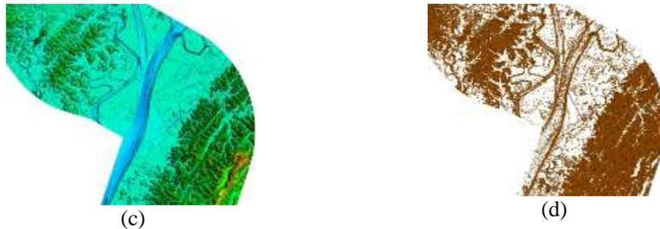
Figure 15. (15a) Ground LiDAR with elevation reference are refer to Benchmark HK.64.09.046, (15b) Bathymetric Data in River Area (Point), (15c) Digital Terrain Model from combination of Ground LiDAR and Bathymetry, (15d) Contour Data derived from DTM in fig. 15c.
