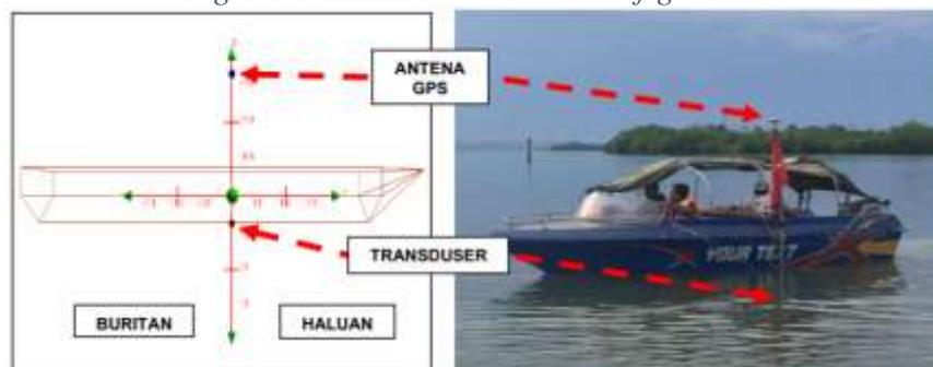
Figure 9. SBES Lever Arm Configuration
