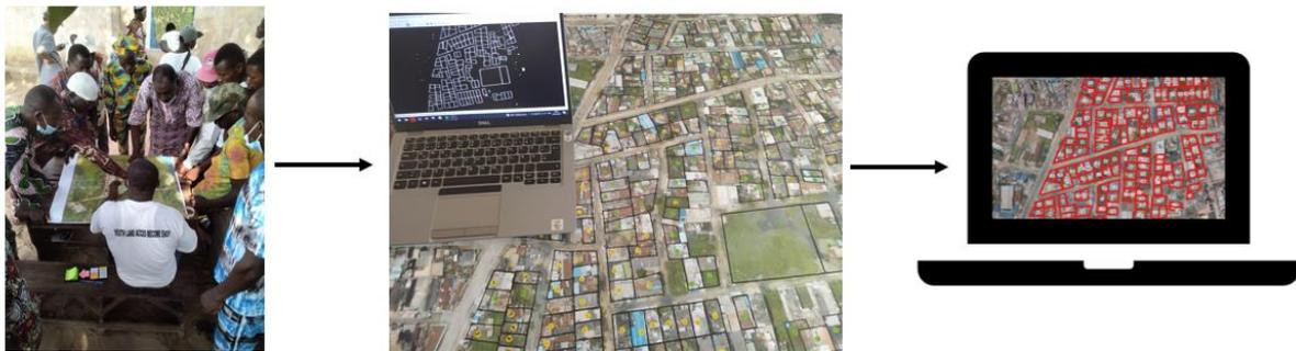
Figure 3: SmartLandMaps digitisation: 1) community mapping to create a sketch map on top of a base map, 2) automatic extraction of sketched lines based on machine learning and computer vision techniques, 3) georeferencing and conversion into GIS vector formats ready to be integrated into existing GIS platforms or land information systems
