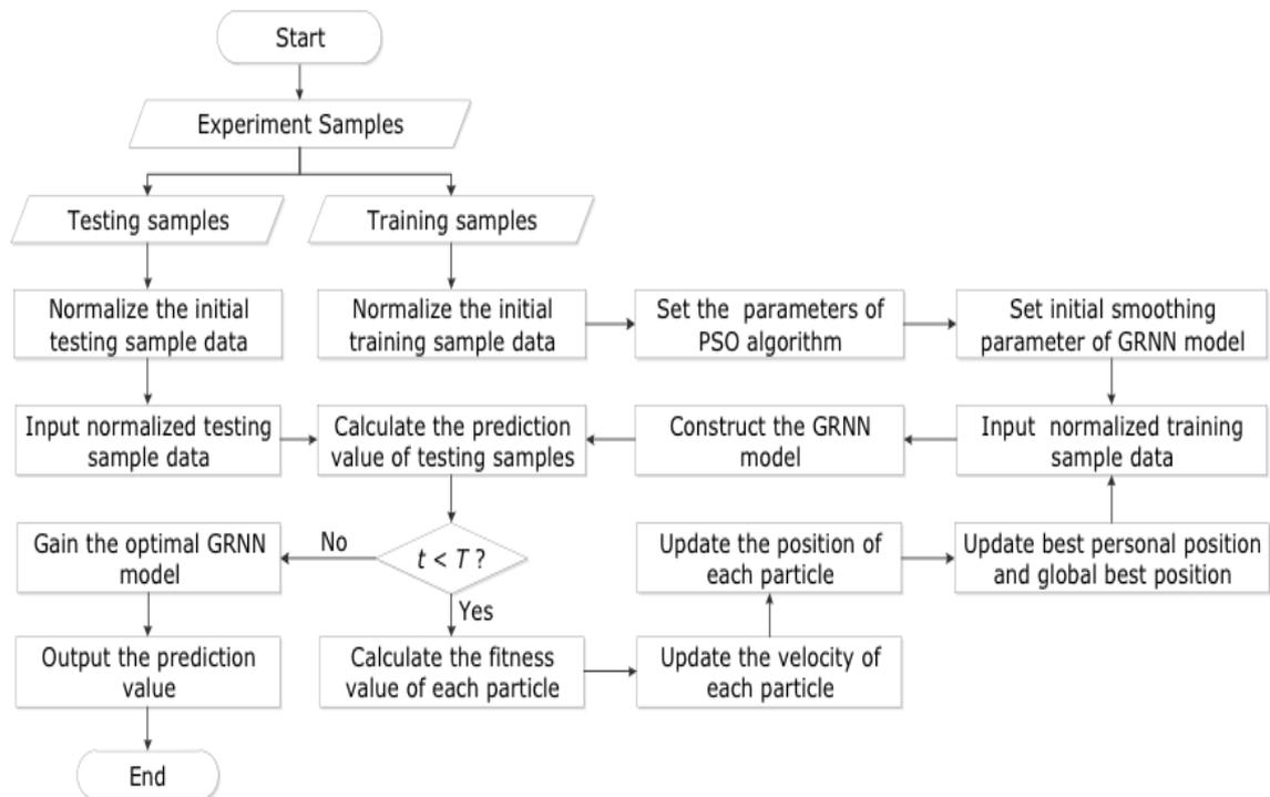
Figure 3 A Flow Chart of a Hybrid PSO-GRNN
