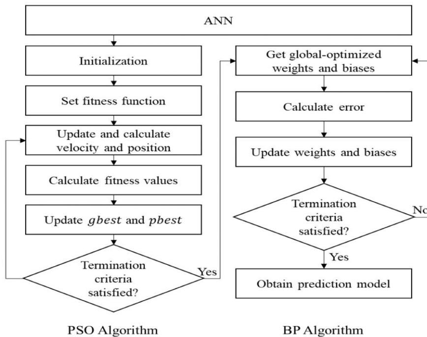
Figure 1 A Flow Chart of Hybrid PSO-BPNN
