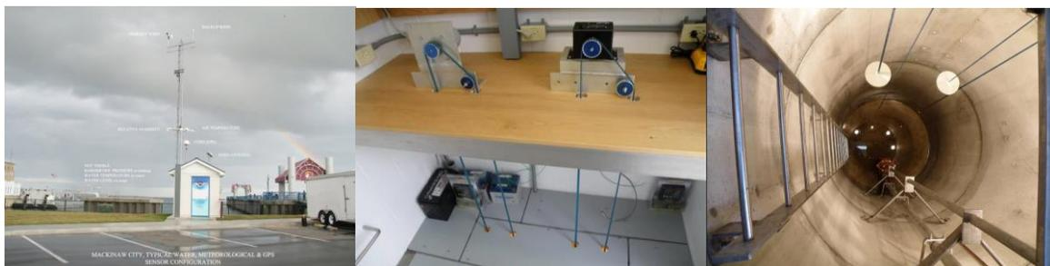
Figure 2 NWLON station at Mackinaw City, MI (courtesy Jeff Oyler, CO-OPS and USACE). Station setup includes numerous antennas including a NOAA CORS Network receiver (left). Inside, measurements are made from the table datum (middle) into the stilling well (right)
