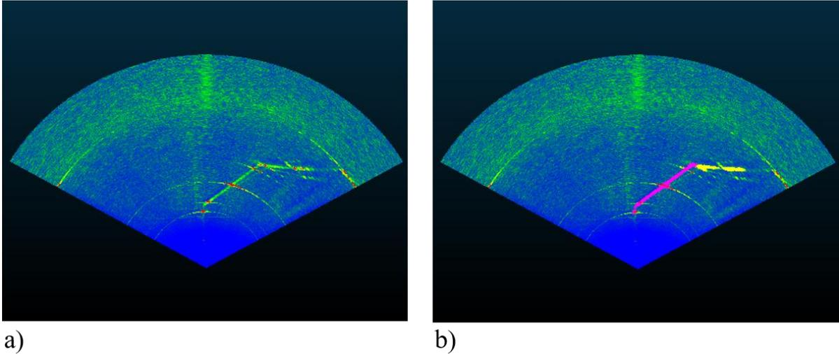
Figure 9: a) Measurement of the seafloor with a pipeline using imaging sonar. b) The pink and yellow highlighted points are respectively segments that were successfully detected as a pipeline by the developed algorithm.
