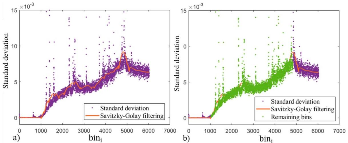
Figure 5: a) The standard deviation calculated for each of the 6032 bins, together with the result of the Savitzky-Golay filtering of order 2. b) Marked in green are the bins determined by the algorithm, which represent the ground measurements.
