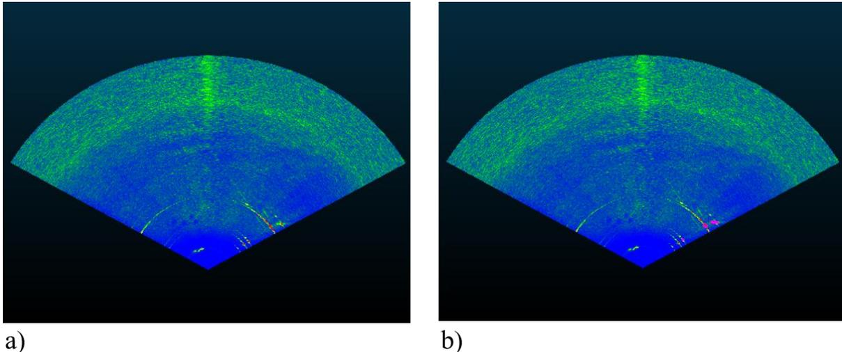
Figure 11: a) Measurement of the seafloor without a pipeline. b) A possible pipeline segment was detected in pink. If a pipeline is searched for by the AUV, the segment can be investigated further by steering the AUV in the direction of the segment.
