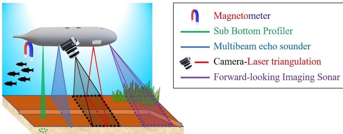
Figure 1: Schematic representation of the various sensor options that can be installed on an autonomous underwater vehicle to enable automatic identification of pipelines in its environment.
