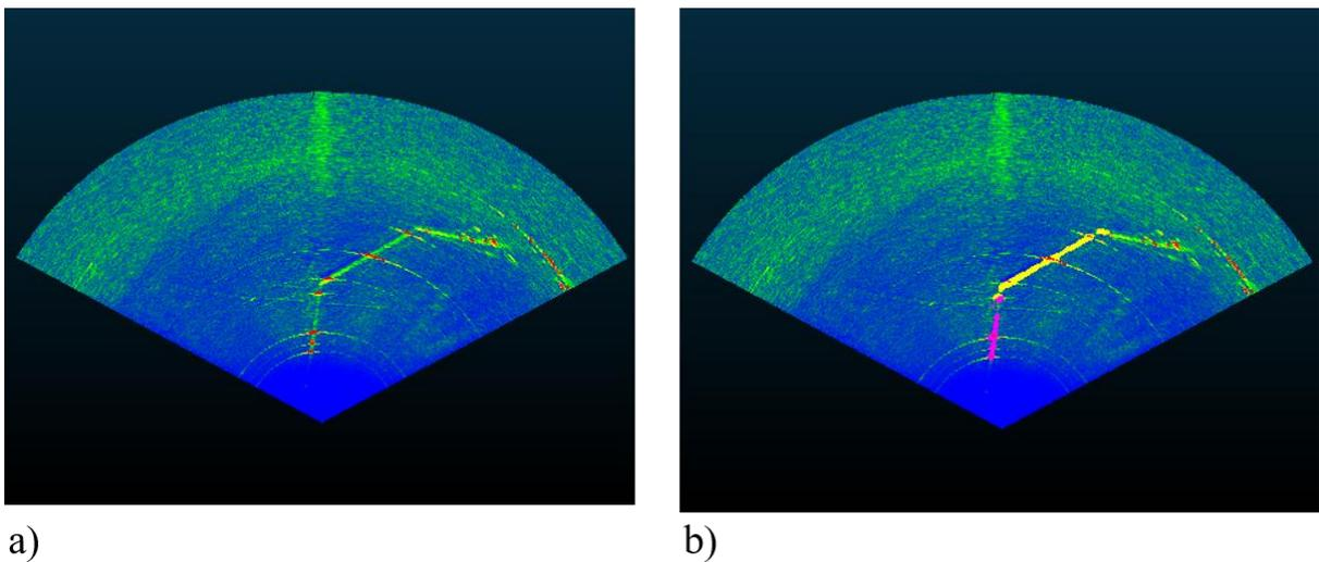
Figure 10: a) Measurement of the seabed on which a pipeline with two branches runs, using imaging sonar. b) The pink and yellow highlighted points are the first two segments that were automatically detected by the algorithm.
