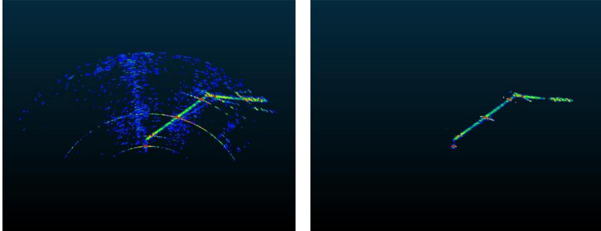
a) Point cloud after filtering out the essential measurement area and applying a statistical outlier removal filter. b) Point cloud after filtering out the essential measurement area and applying a statistical outlier removal filter and additionally a radius outlier removal filter.
