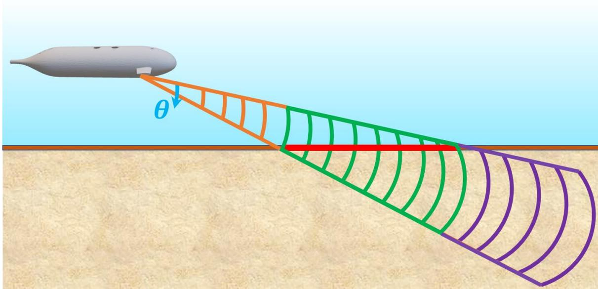
Figure 3: This schematic shows a side view of a measurement taken with an imaging sonar aimed at the seabed. The orange bins do not contain any crucial information for detecting pipelines, while the green bins represent the important measurement area that includes information about the seafloor and potential pipelines located there. For the purple area, the entire signal has already been reflected away from the seafloor, making accurate measurements impossible.
