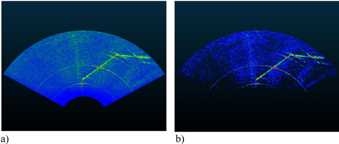
Figure 6: a) Point cloud with ground measurements, where irrelevant areas were automatically filtered out using the standard deviation of the bins and the elaborated method. b) Point cloud after filtering out points with low measured intensity.
