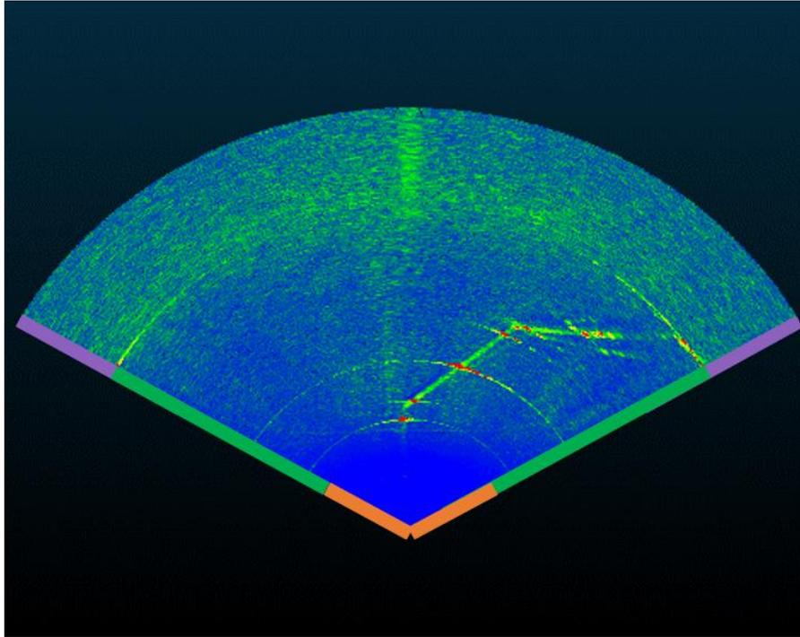
Figure 4: A measurement from an imaging sonar. In addition to the pipeline, the three areas are also visible. These are marked on the sloping sides of the measurement with the respective colors. The green area represents the measurement of the sea bottom, while the orange area indicates the space between the sensor and the sea floor. The purple area represents the theoretical measurement of the ground, which cannot be directly measured due to the non-penetrating signal.
