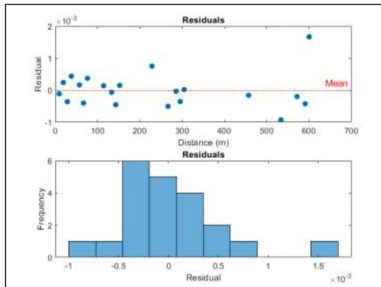
Figure 8: Residuals from adjustment of measured test line distances.
