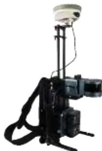
**Figure 6 Cygnus backpack mobile laser scanning system**
