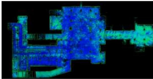
**Figure 3 Point cloud slice effect of underground parking lot**
