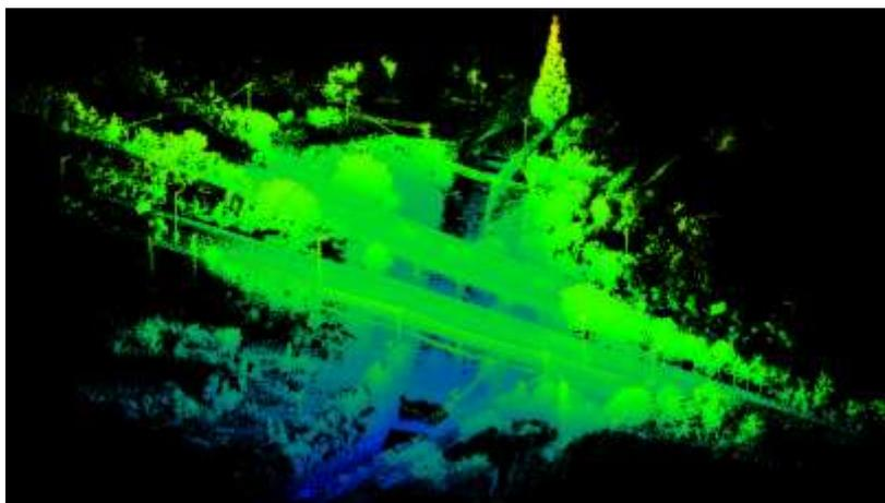
**Figure 7 Backpack scanning point cloud data**
