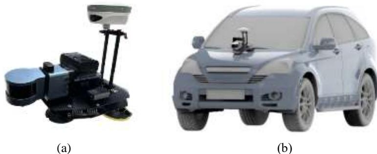
**Figure 9** Car kit of the Cygnus SLAM scanner
