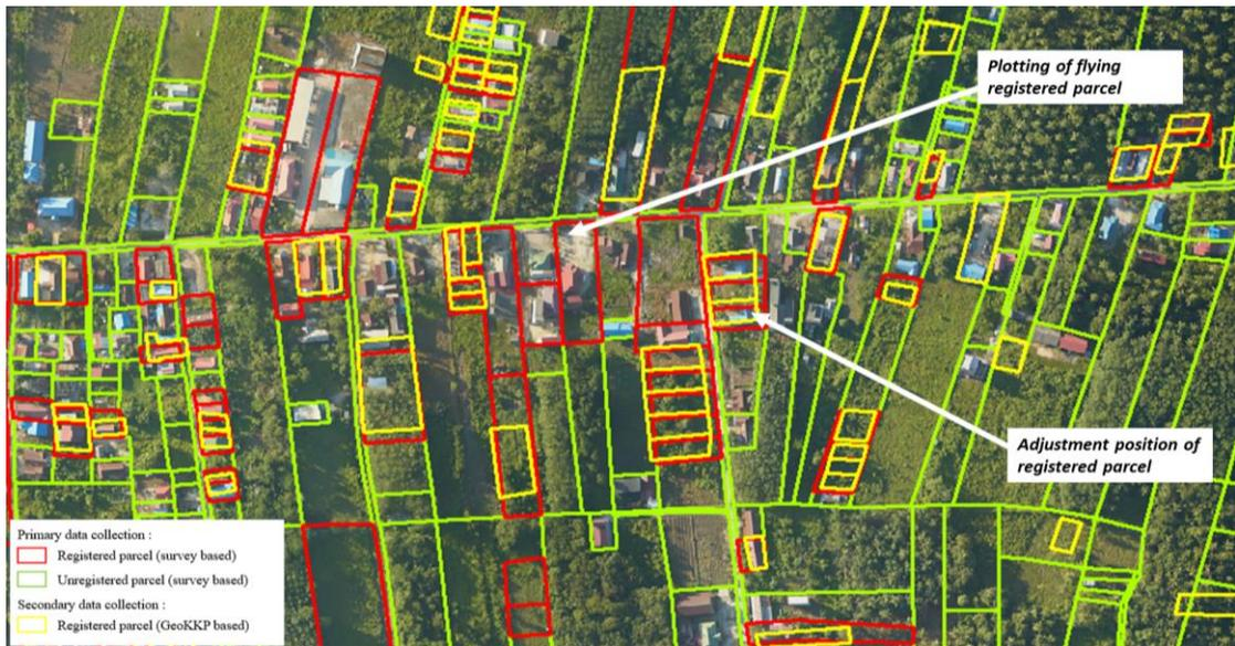
Picture 12: Discrepancy of registered parcels in GeoKKP with the existing condition
