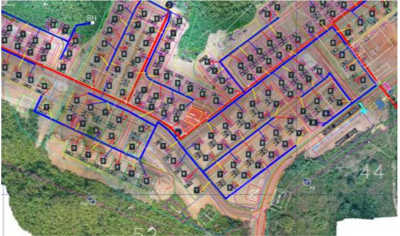
Fig. 22: CAD Design Overlaid on Drone DEM to Check Compatibility
