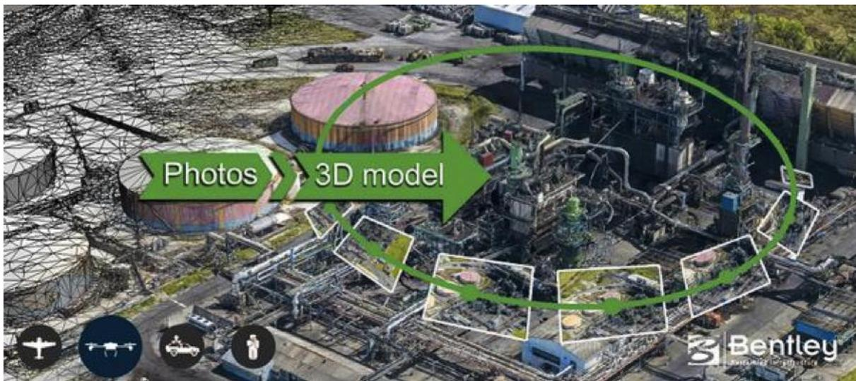
Figure 3: Wide area mesh form of Digital Twin is generally limited to planning and conceptual design applications
