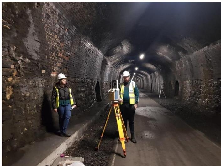
*Figure 3 Image showing the offset from the wall for scanners and targets (Anderson, 2022)*
