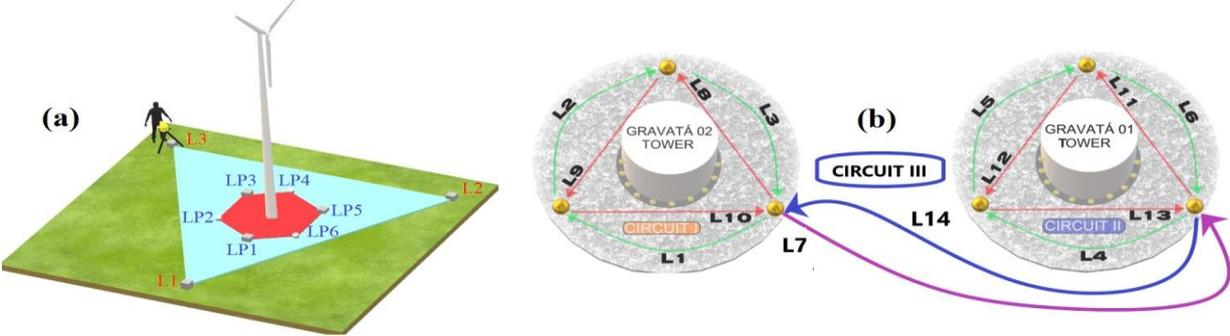
Figure 04 – Geometric configuration of the geodetic network
