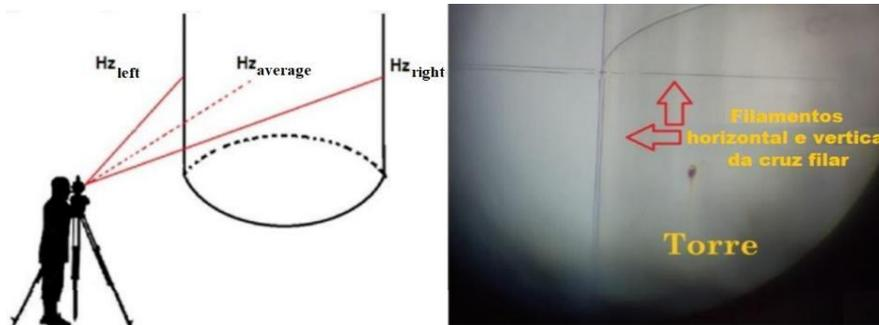
Figure 07 – Method of measuring edges.
