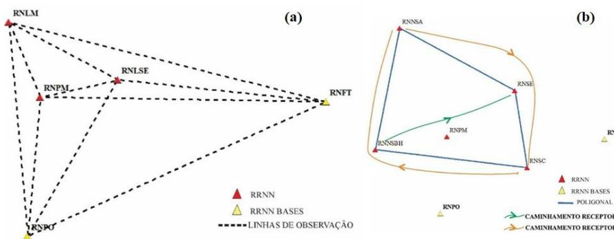
Figure 13 - Schematics of the surveys carried out in the second campaign. (a) first stage (b) Second stage.
