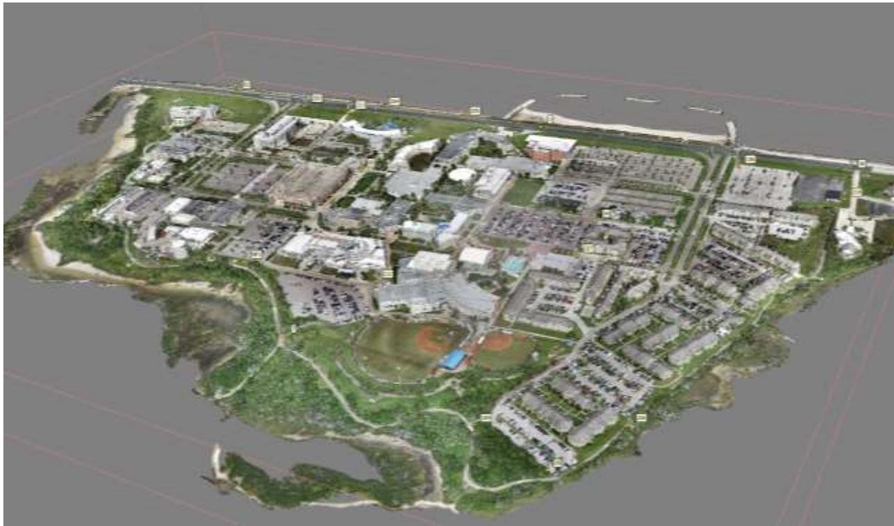
Fig: Colorized 3D point cloud.
