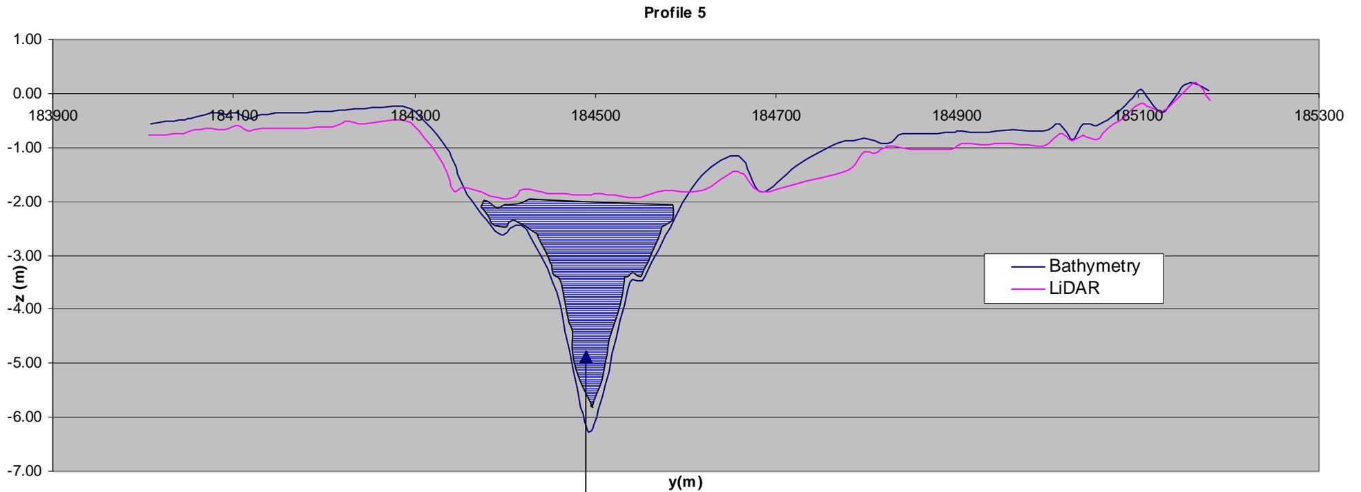
Navigation Channel – This demonstrates the non-water penetrating nature of LiDAR when compared to bathymetry data collection.
