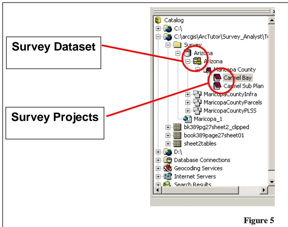
Survey computations are performed on data within survey projects to resolve the survey computation network and compute coordinates for the surveyed points. The results can be displayed in the GIS systems map space for GIS editing, figure 6.
